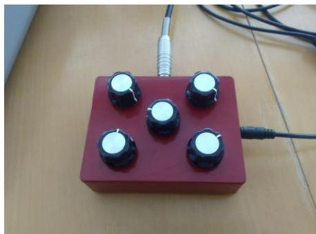
2) I built a wave generator that produces sound waves from 1Hz to 1MHz, to be able to experiment with the recording of infrasound and pitch shifters to compose music.
